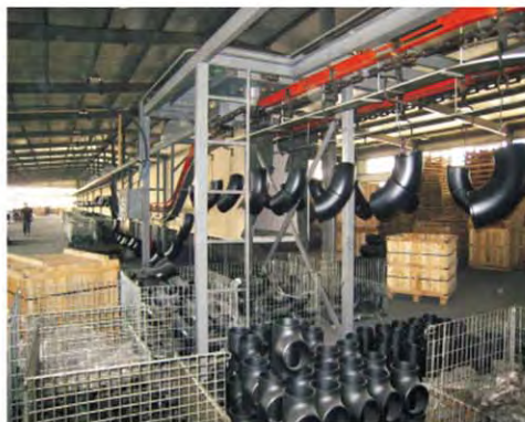
Advanced BW Fittings Painting Line
